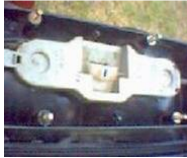
rear of tail-light showing globe holder
